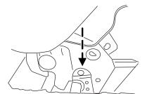
3. Lower back of seat onto the rear tubs until both release controls latch into place. Be sure that the seat is locked in place both front and back.
